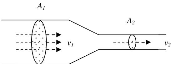
The area of the pipe on the left side is  $A_1$ , and the speed of the fluid passing through  $A_1$  is  $v_1$ . As the pipe tapers to a smaller area  $A_2$ , the speed changes to  $v_2$ . Since mass must be conserved, the mass of the fluid passing through  $A_1$  must be the same as the mass of the fluid passing through  $A_2$ . If the density of the fluid is  $\rho_1$ , and the
