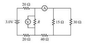
In the circuit shown above, the current through the ammeter is 20 mA and the voltmeter indicates 1.0 V.
