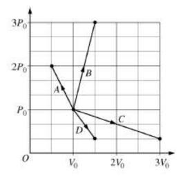
48. Identical samples of gas initially have pressure P<sub>0</sub>, volume V<sub>0</sub>, and temperature T<sub>0</sub>. In some experiments, students take samples through each of the processes shown in the graph above. The final temperature is equal to the initial temperature for which of the processes? Select two answers.
